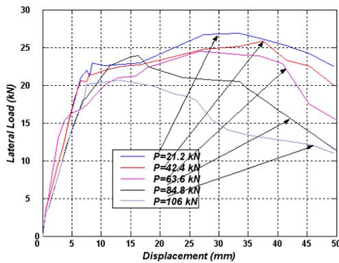
**Figure (7): Capacity curves for unreinforced columns designed according to ACI (Pre-1971)**
