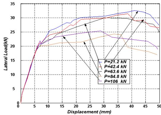
**Figure (8): Capacity curves for retrofitted columns designed according to ACI (Pre-1971)**
