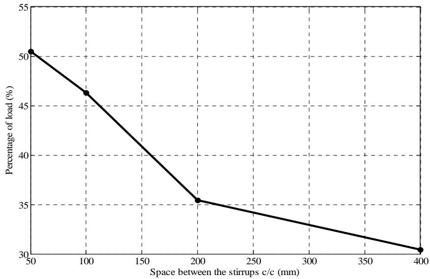
**Figure (12): The percentage of increasing load capacity for shear capacity cases**
