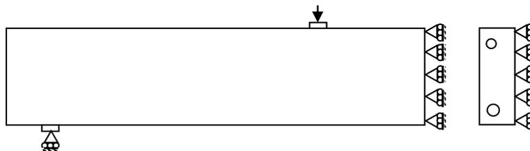
Figure (3): Boundary conditions used in numerical work
