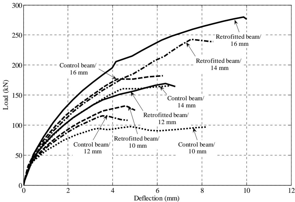
**Figure (7): Load *versus* mid-span deflection for internal tensile reinforcement models**
