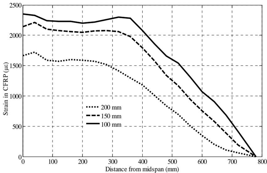
Figure (18): Axial strains in CFRP layer for beam width
