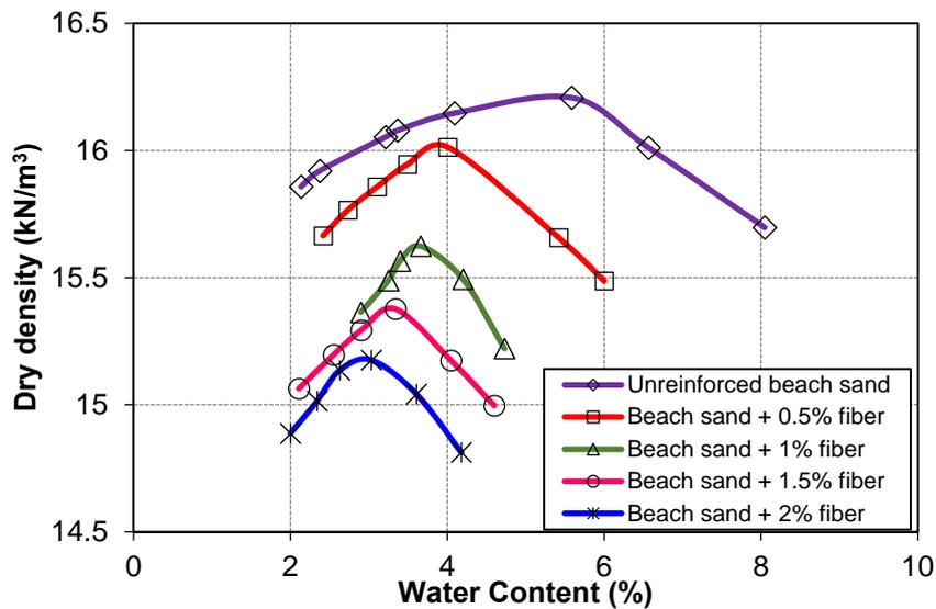
Figure (4): Effect of fibres on proctor compaction curves
