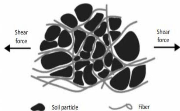
Figure (3): Interfacial mechanism between soil and fibres
