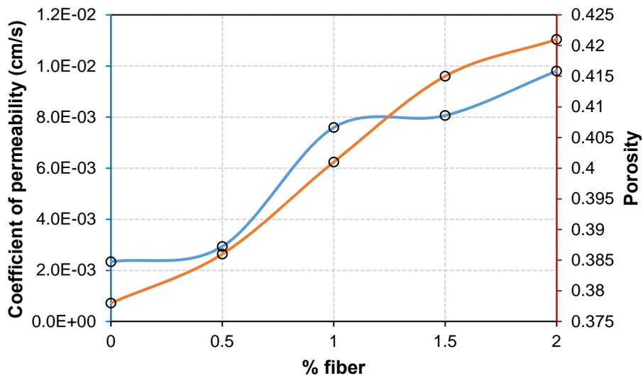
Figure (7): Effect of fibres on permeability and porosity
