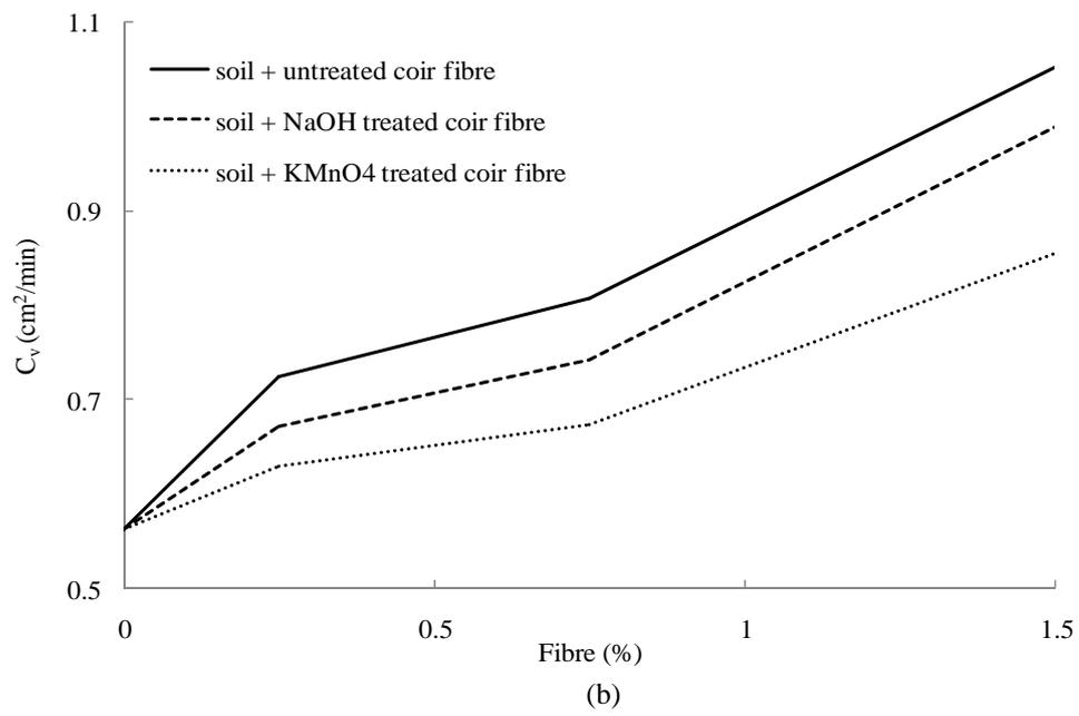
**Figure (11): Variation of coefficient of consolidation with fibre percentage for (a)  $\Delta\sigma = 98$  kPa and (b)  $\Delta\sigma = 392$  kPa**
