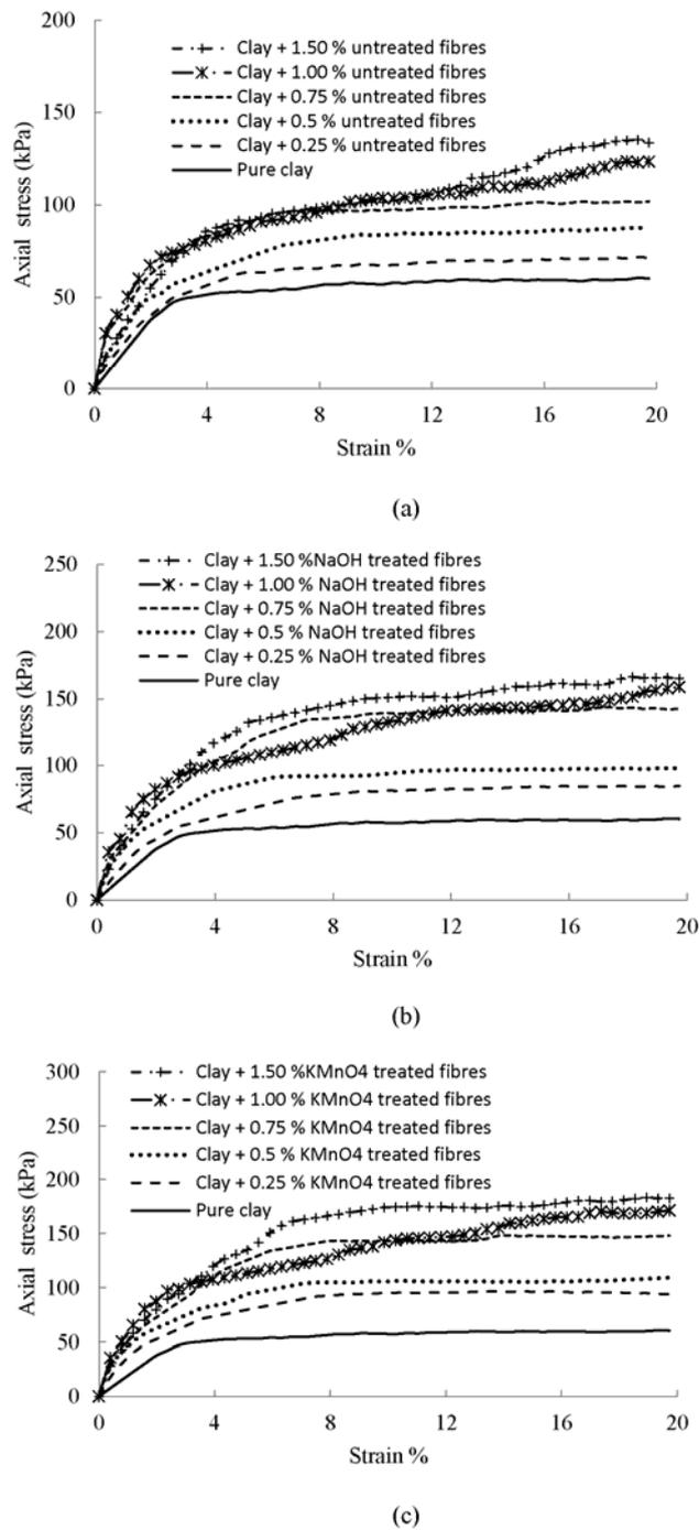
Figure (4): Variation of axial stress with fibre percentage for soil reinforced with (a) untreated fibres, (b) NaOH-treated fibres and (c) KMnO<sub>4</sub>-treated fibres ( $S_r \cong 100\%$ )
