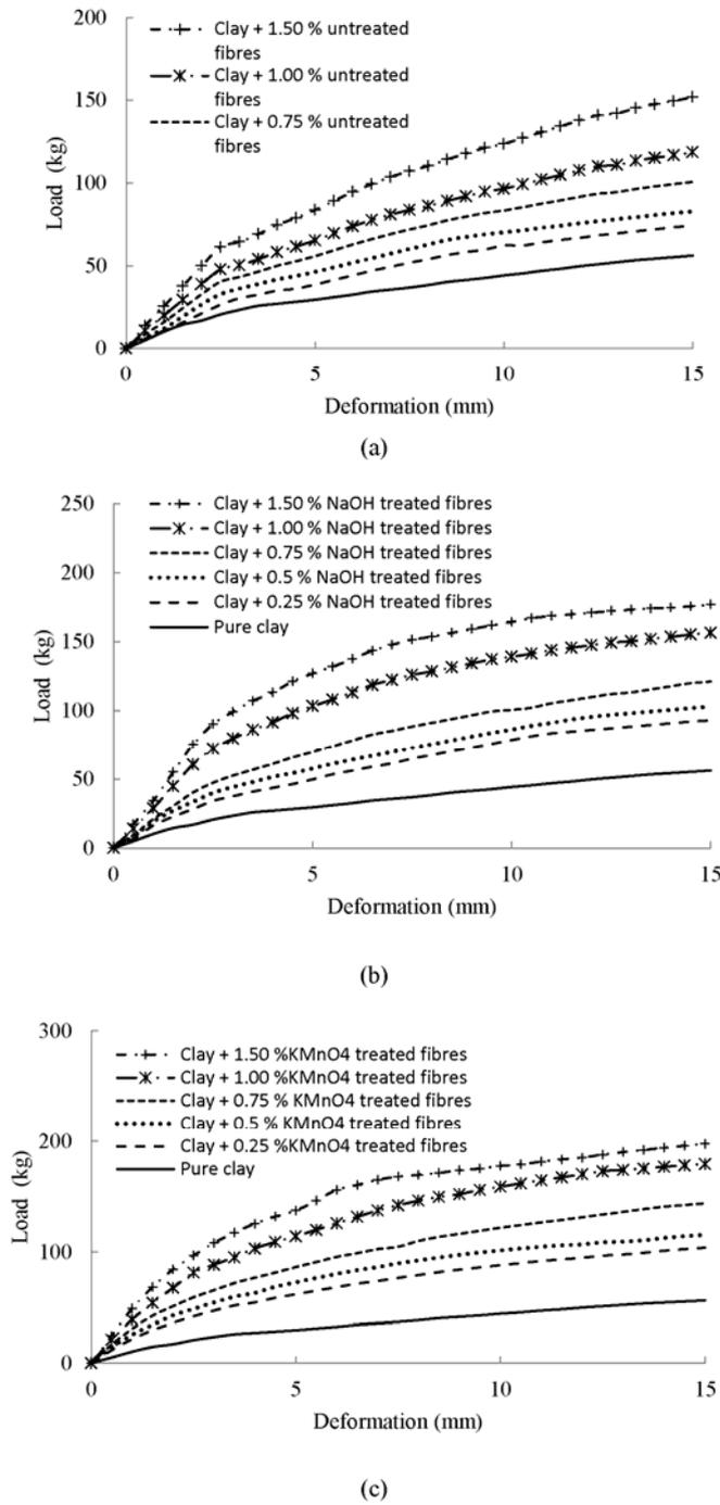
**Figure (9): Load deformation behavior for soil reinforced with (a) untreated fibres, (b) NaOH-treated fibres and (c) KMnO<sub>4</sub>-treated fibres (Sr $\cong$  100%)**
