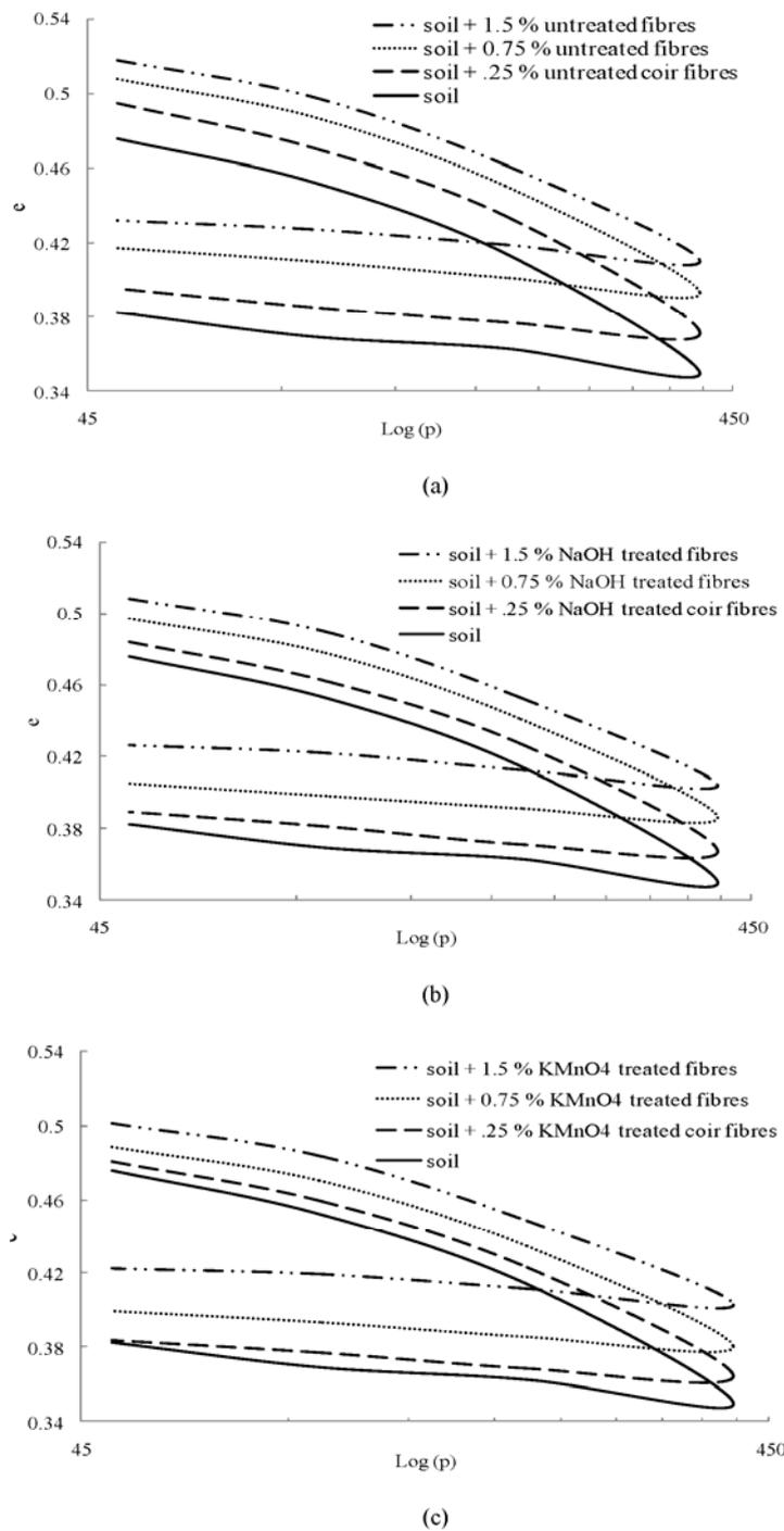
Figure (12): Pressure-void ratio curves for soil reinforced with (a) untreated fibres, (b) NaOH-treated fibres and (c)  $\text{KMnO}_4$ -treated fibres
