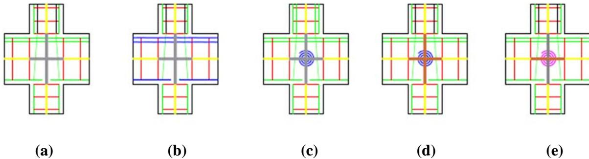
**Figure (5): (a) Centerline joint model (CLM), (b) scissors model without rigid links (SM), (c) scissors model with rigid links (SML), (d) centerline model with reduced beam flexural capacity (CLRBM) and (e) ASCEM model**
