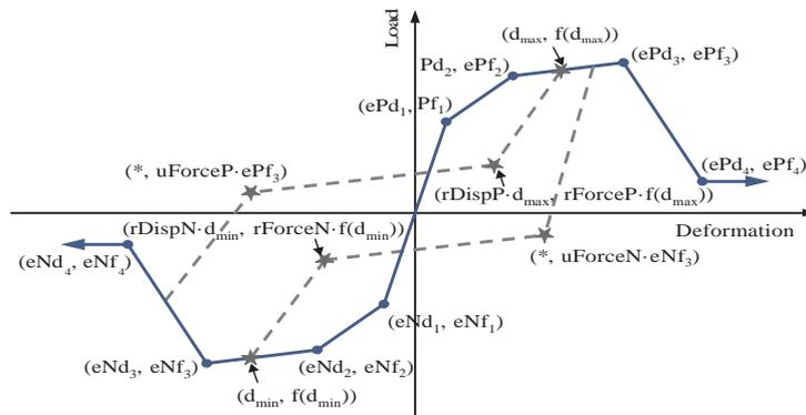
**Figure (2): Pinching 4 damage material model**
