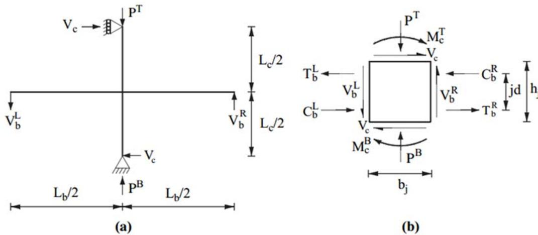
Figure (4): The free body diagrams of (a) a typical interior beam-column joint test setup and (b) its joint panel
