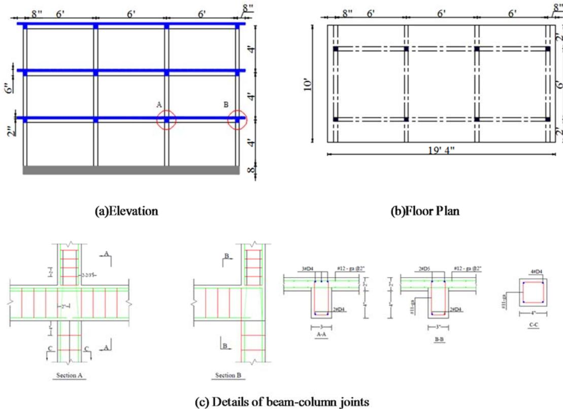
**Figure (6): Details of prototype frame and sub-assemblages**
