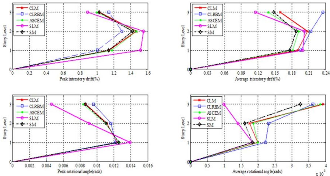
**Figure (10): Drift ratio and rotational demand for the various joint models**
