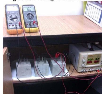
Figure (6): Electrical testing photos showing resistivity measurements
