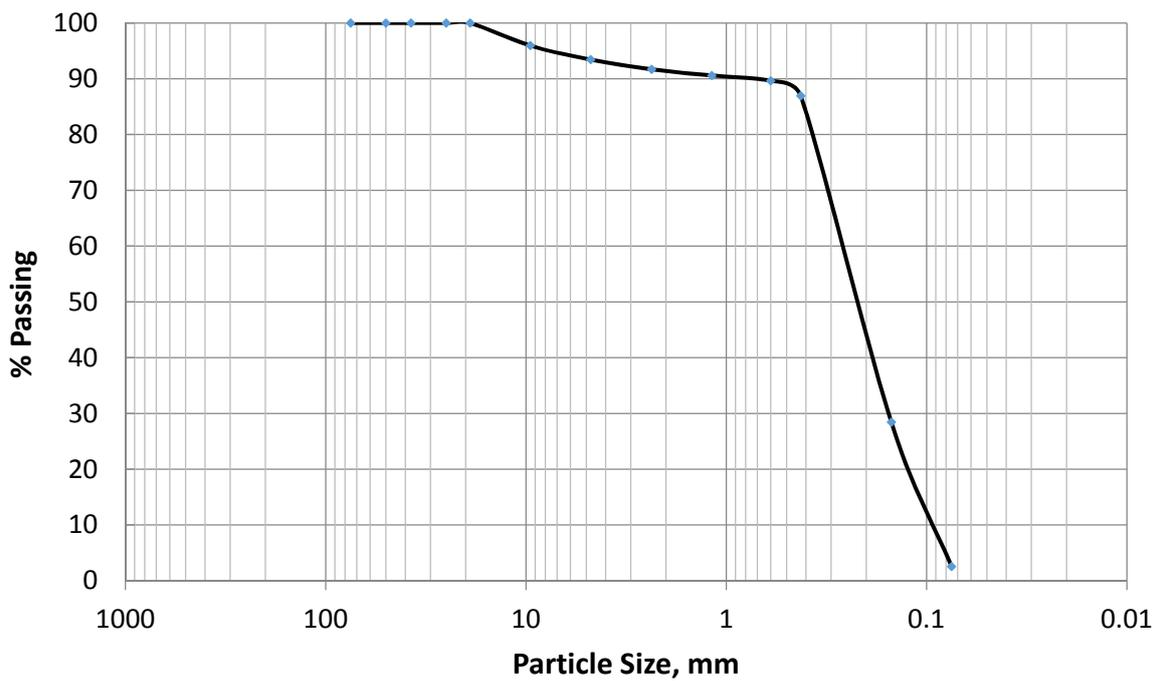
**Figure (1): Grain size distribution of the soil in the site**
