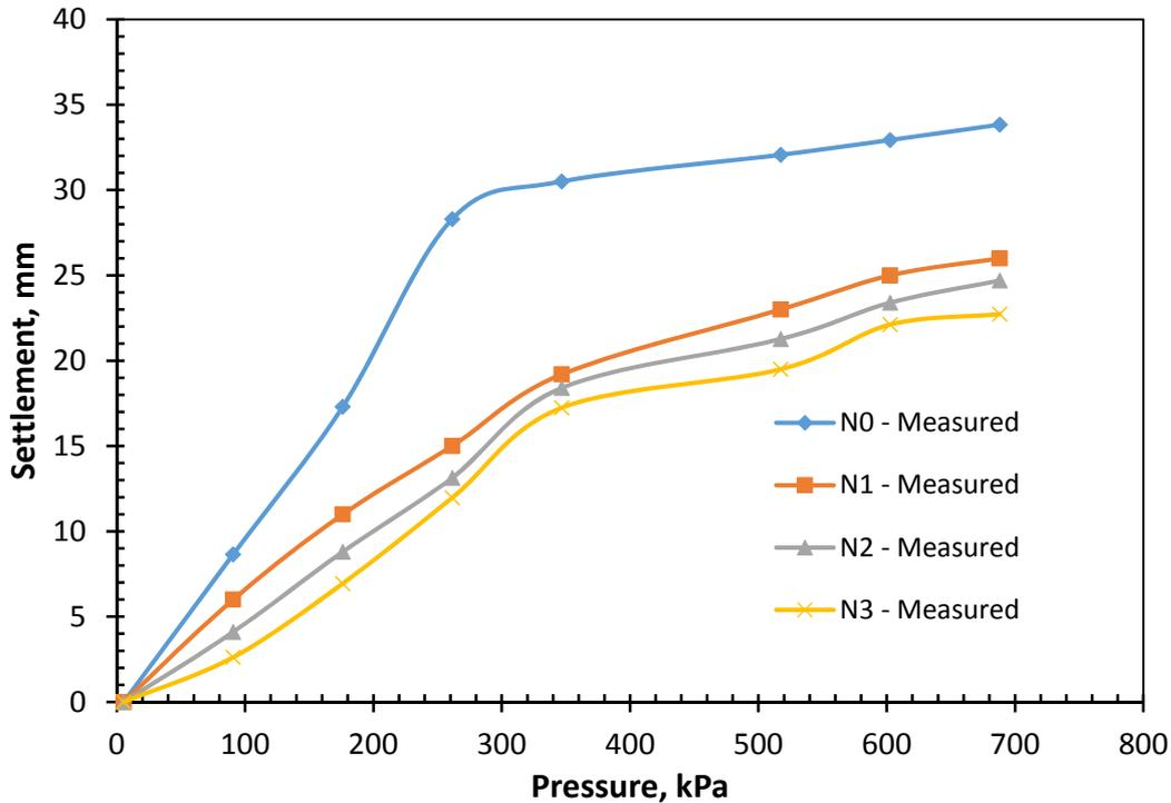
**Figure (7): Plate load pressure-settlement response at the surface for unreinforced soil and reinforced soil at different depths**
