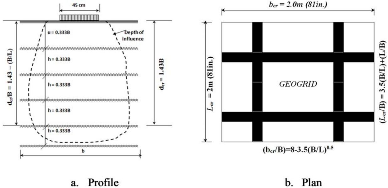
**Figure (5): Depth of influence of geogrid reinforcement**
