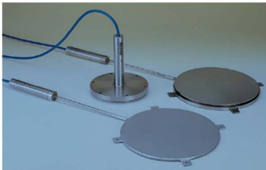
**Figure (6): Earth pressure cell model 4800 (Geokon, Inc.)**
