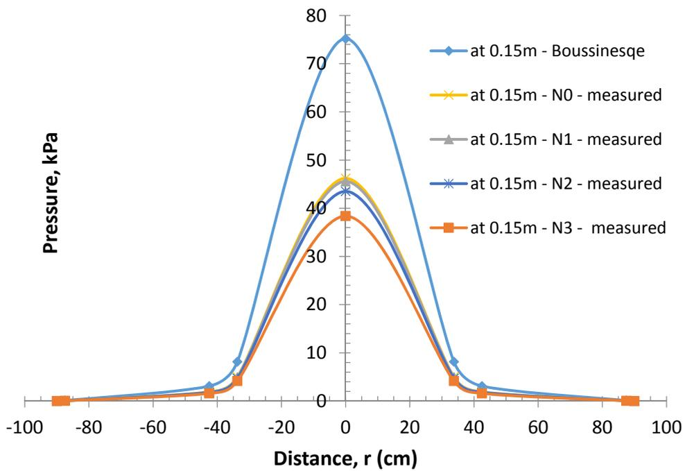
Figure (10): Comparison between measured and calculated stresses (using Boussinesq) in horizontal plane at a depth of 0.15 m of unreinforced and reinforced soil (applied pressure = 90.7 kPa)
