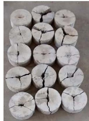
**Figure (12): Failure pattern on final impact failure**
