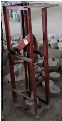
**Figure (11): Modified drop impact testing machine**
