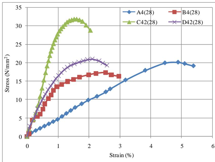
**Figure (3): Stress-strain characteristics of fresh/ C & D aggregate concrete without/with glass waste (with superplasticizer and fiber)**
