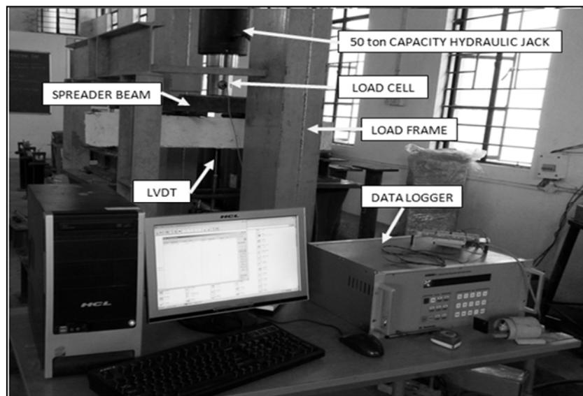
Figure (3): Test setup of SCS composite beam
