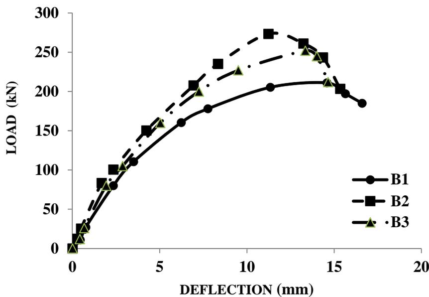
**Figure (4): Load vs. deflection for composite beams**
