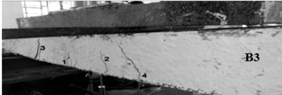
Figure (7): Flexural cracks in composite beam B3
