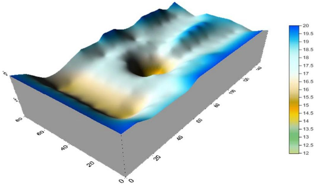
Figure (10): Bed bathymetry for experimental run A4 (scale in cm)
