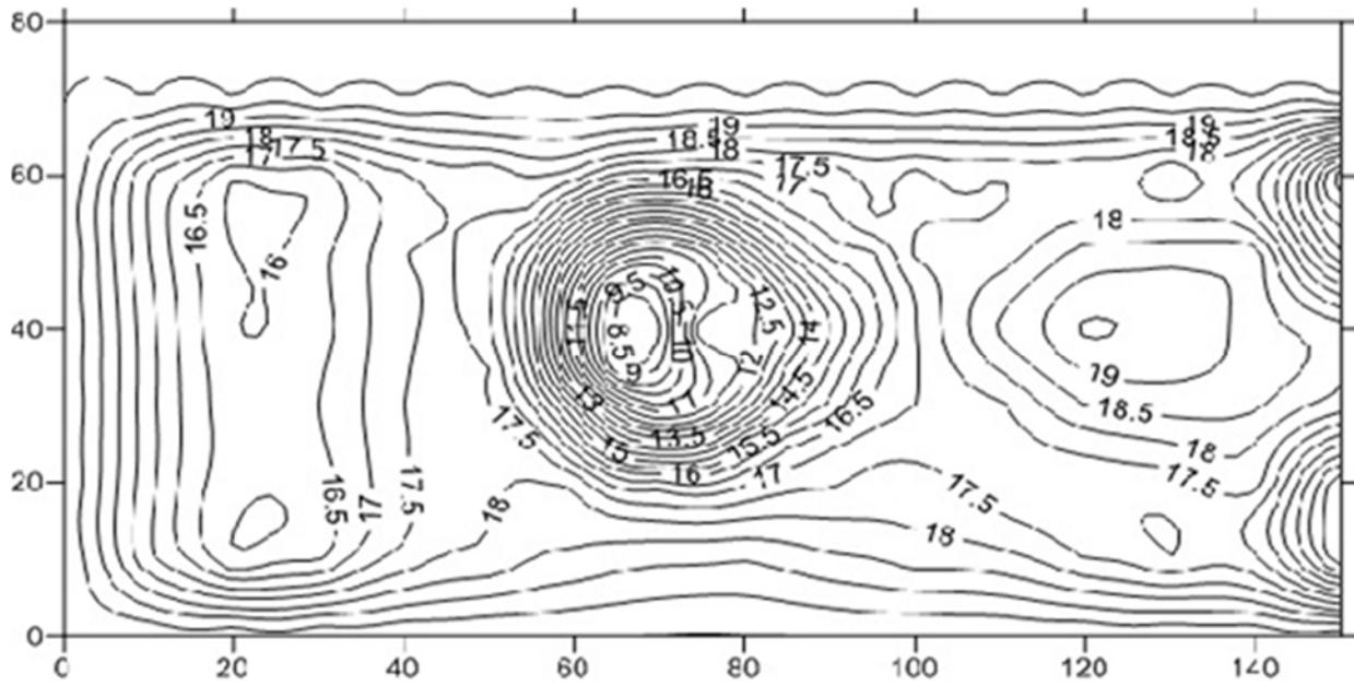
Figure (14): Graph of topographic bed for experimental run C4 (scale in cm)
