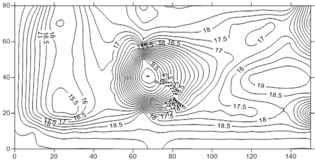
Figure (13): Graph of topographic bed for experimental run B4 (scale in cm)
