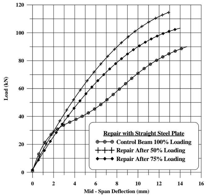
Figure (10): Effect of straight steel plate repair
