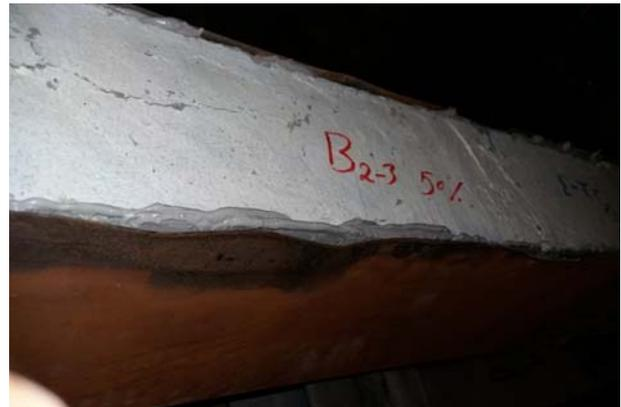
(c) Debonding of steel plates and crushing of concrete at the load points of beam B2-3
