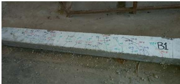
**Figure (4): Control beam (B1) after failure**
