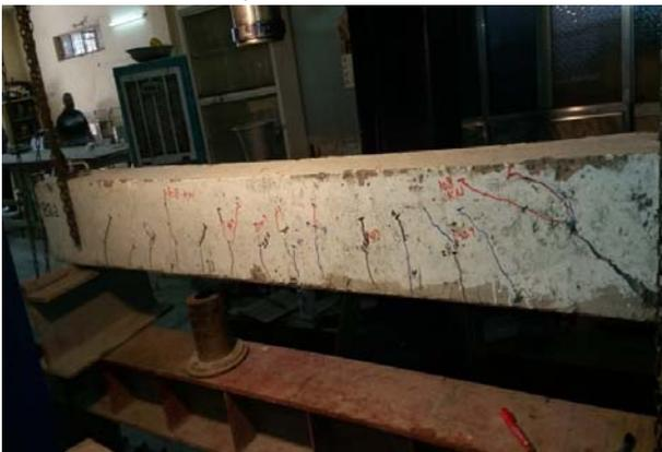
(b) Flexural and shear failure of beam B2-2
