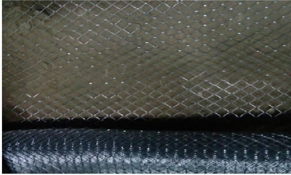
Figure (1): Ferro-mesh used in the present study
