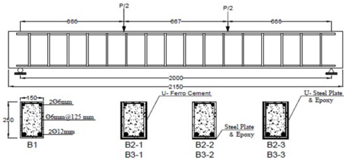
**Figure (2): Details of reinforcement of the tested beams**
