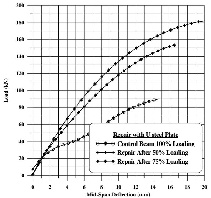
Figure (11): Effect of U-steel plate repair
