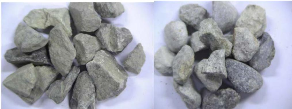
**Figure (1): The coarse aggregates used in this study; (a) natural coarse aggregate (NG), (b) recycled coarse aggregate (RG)**
