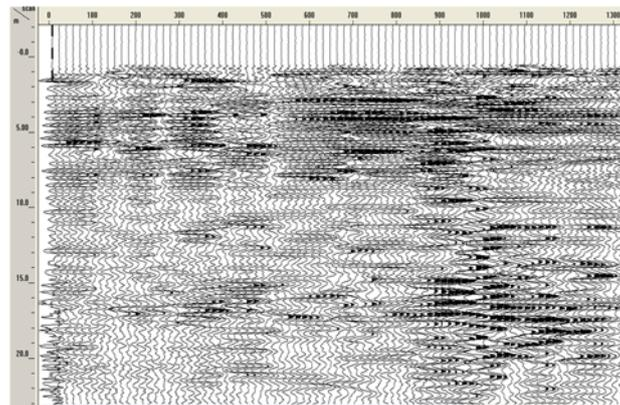
Figure (5): Wiggle waveform of GPR
