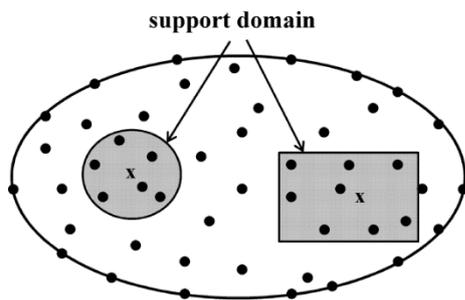
**Figure (1): Representation of support domains which are used for interpolation**
