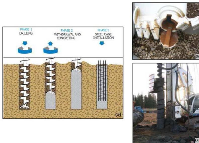
**Figure (11): Schematic drawing of CFA pile construction**
