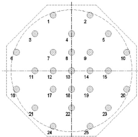
Figure (12): Piles' disposition under the tank floor
