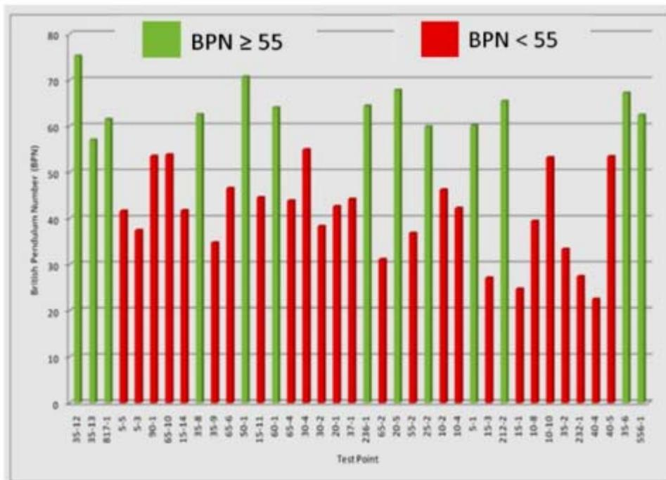
**Figure (8): Obtained British pendulum numbers for all test locations**
