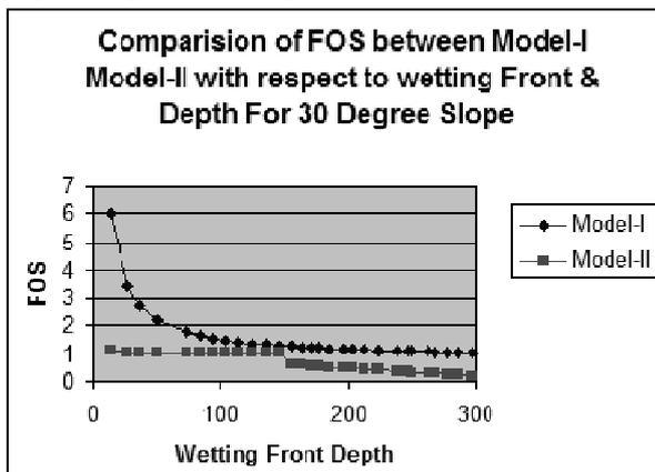
**Figure (5): Variation of FOS with wetting front depth for model-I and Model-II**
