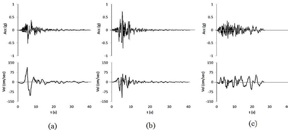
**Figure (3): Pulse type ground motion records (a) 1979 Imperial Valley (El Centro Array #4) [IV79] and (b) 1994 Northridge (Newhall, Fire Station) [NR94] and non-pulse-type record (c) 1980 Victoria Mexico (Chihuahua) [VM80]. Acceleration time histories of the selected records are shown in the top row and velocity time histories are shown in the bottom row (Pacific Earthquake Engineering Research Center, 1014)**
