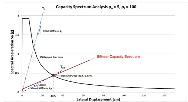
**Figure (2): Example capacity spectrum analysis (ATC, 1996)**
