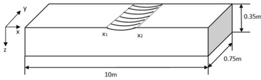
**Figure (1): Model of subgrade during vibrating compaction**
