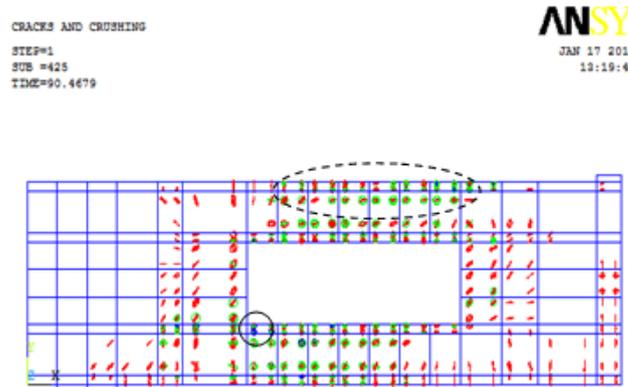
**Figure (20): Crack pattern at a load of 90 kN for beam BS9**
