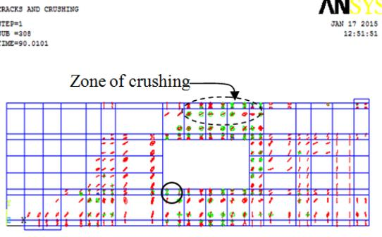
**Figure (15): Crack pattern at a load of 90 kN for beam BS2**
