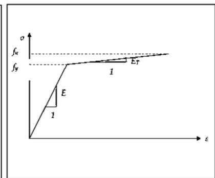
**Figure (3): Uniaxial stress-strain relation for steel**
