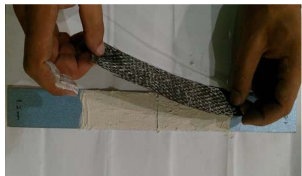
Figure (6): Specimen with applied adhesive
