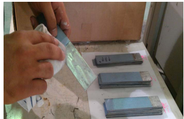
Figure (3): Cleaning with cotton after surface
