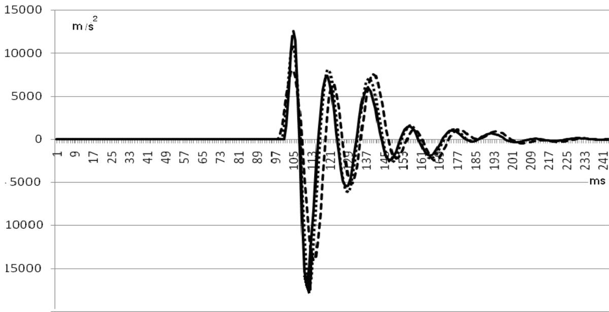
**Figure (4): Acceleration of rail in wheel flat point for different velocities**
