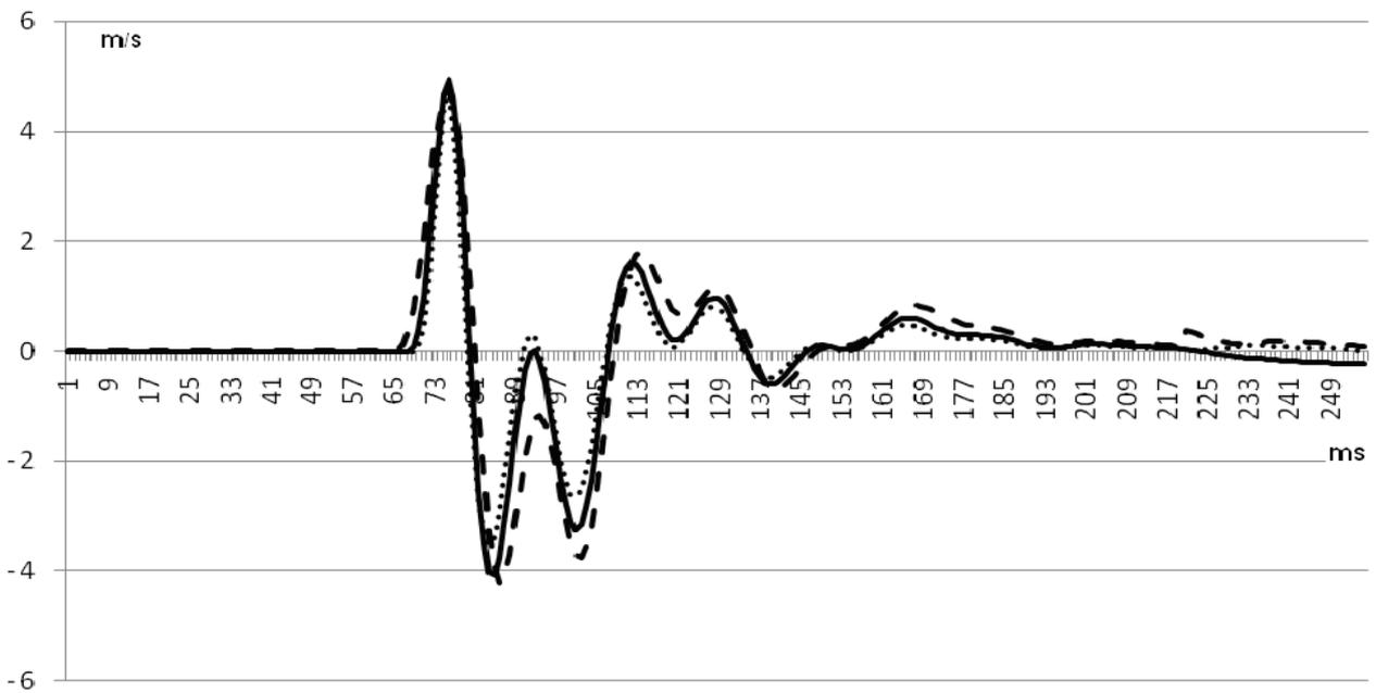
**Figure (5): Velocity of rail in wheel flat point for different velocities**
