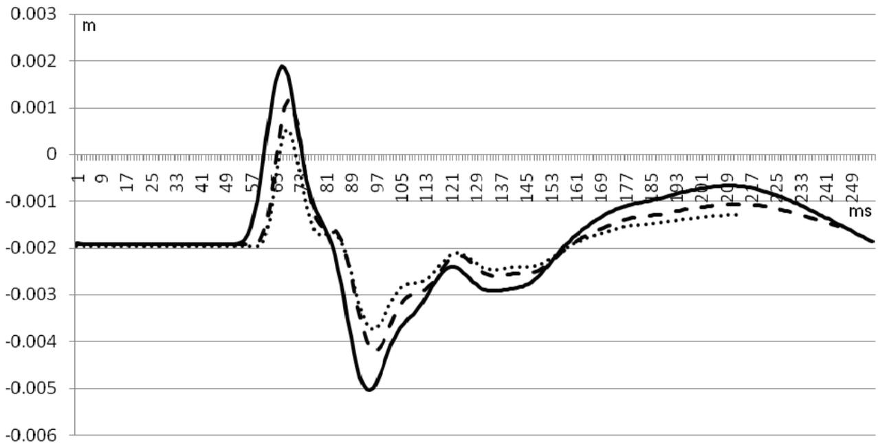
Figure (6): Displacement of rail in wheel flat point for different velocities
