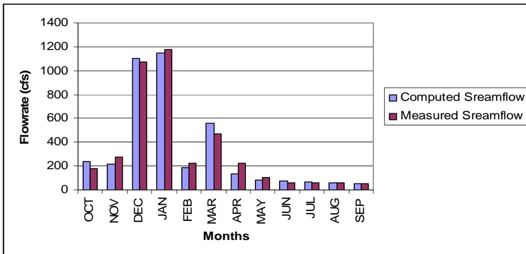
**Figure (3): Comparison between monthly totals of synthesized and recorded flowrate for the water year 2003/2004**
