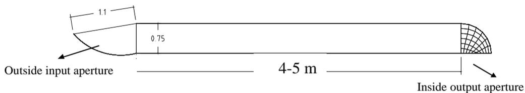
**Figure (3): The tested and simulated anidolic system**
