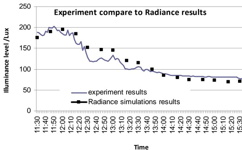
Figure (8): Experimental results compared to radiance simulation in the daylighting chamber
