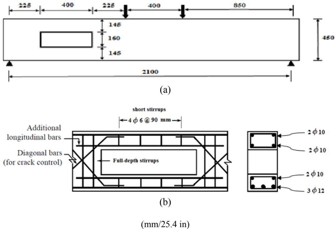
Figure (3): Beam description (a) Opening location (b) Steel reinforcement at the opening
