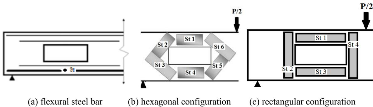
Figure (2): Locations of strain gauge
