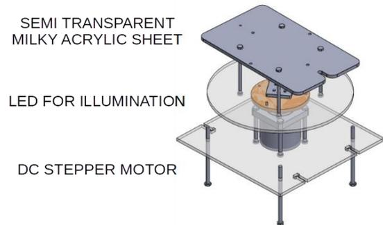
Figure (3): The turntable arrangement
