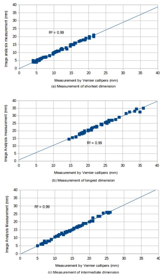
**Figure (8): Comparison of dimensions measured through manual and digital modes**
