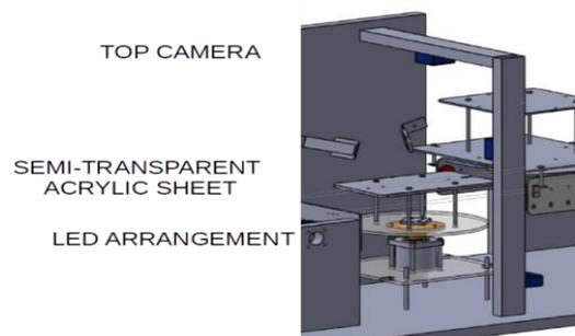
Figure (4): The illumination arrangement
