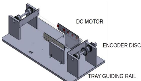
**Figure (5): The conveyor arrangement**
