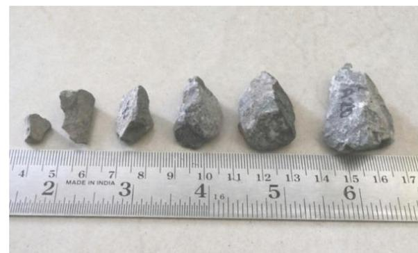
**Figure (2): Various dimensions of aggregates**
