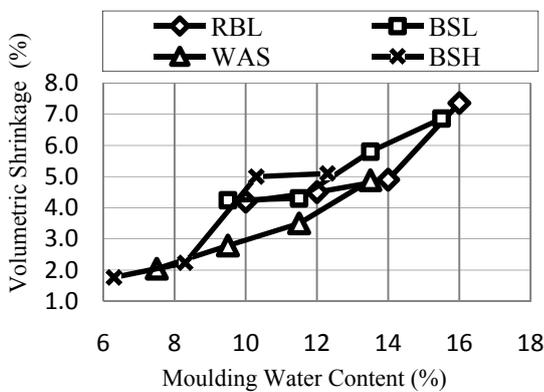
**Figure (4): Variation of volumetric shrinkage strain with moulding water content for the natural soil**
