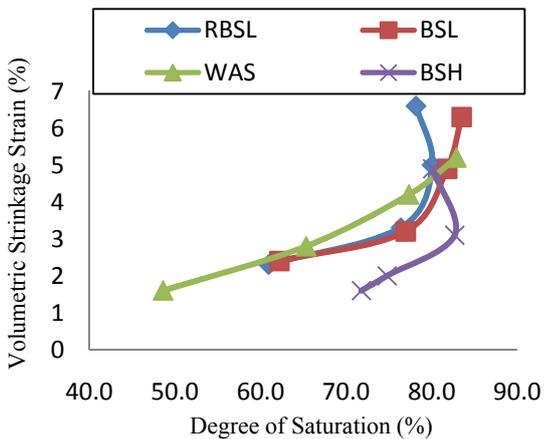
**Figure (11): Variation of volumetric shrinkage strain with degree of saturation for 4% bagasse ash treatment**
