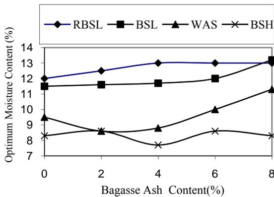
**Figure (3): Variation of optimum moisture content of foundry sand with bagasse ash content**
