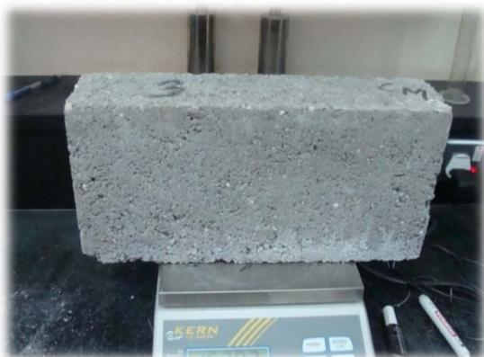
Unit Weight -ASTM C127
