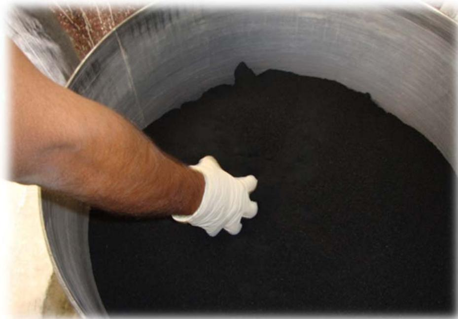
Figure (1): Crumb Rubber Sample
