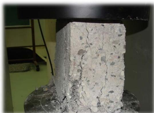
Compression test-ASTM C140
