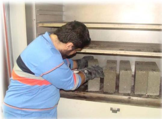
Water Absorption -ASTM C127
