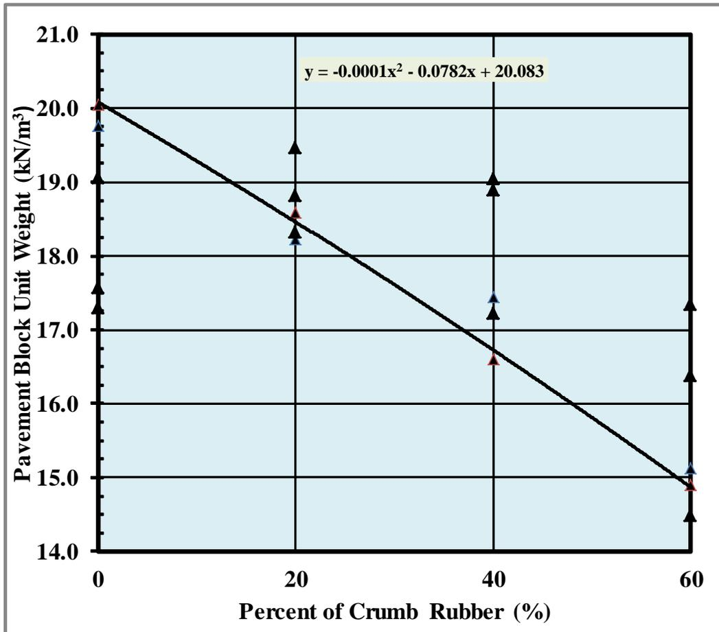
Figure (5): Unit Weights of Crumb Rubber Concrete Pedestrian Blocks
