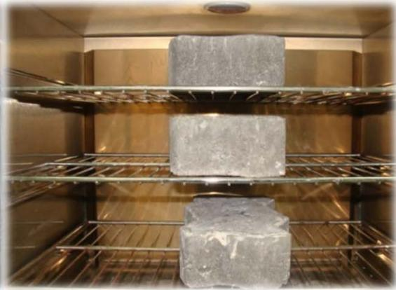
**Water Absorption -ASTM C127**
