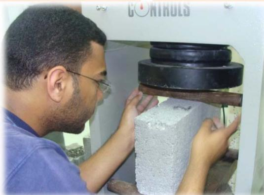
Flexural Test-ASTM C78-02
