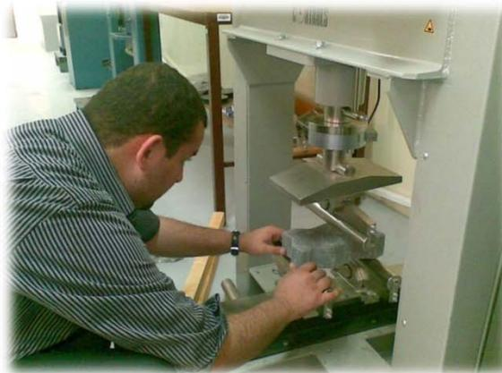
**Flexural Test-ASTM C78-02**
