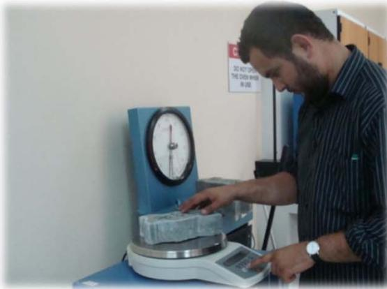
**Unit Weight -ASTM C127**
