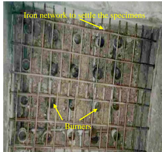
Figure (3): Brick stove of net methane burner
