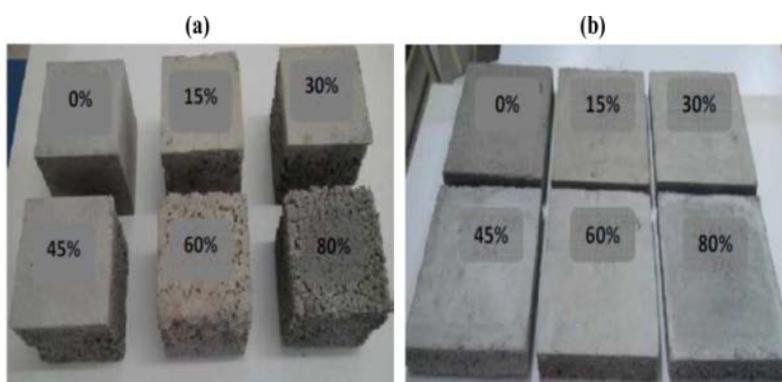
**Figure (1): Cubic specimens (a), parallelepiped specimens (b)**
