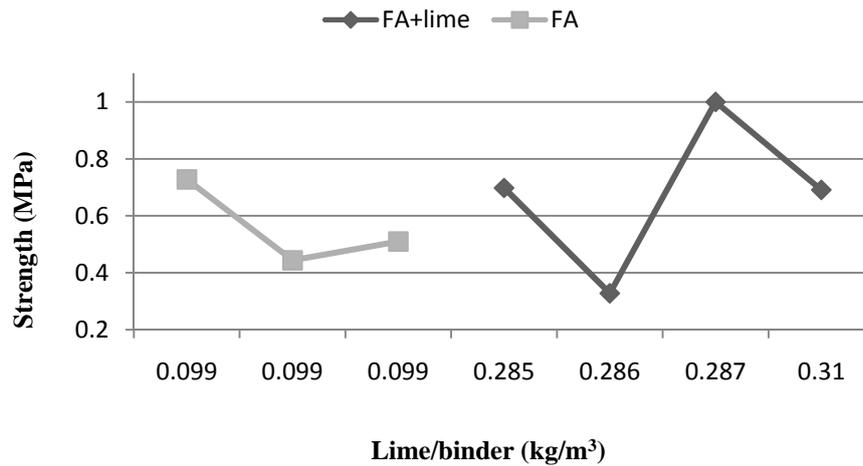
Figure (18): Relationship between compressive strength and lime/binder
