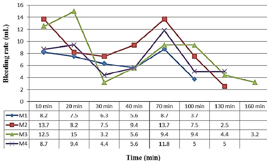
Figure (5): Relationship of bleeding versus time (M1-M4)
