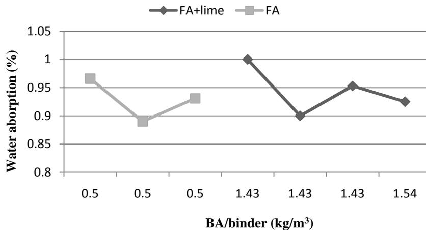
Figure (17): Relationship between water absorption and BA/binder
