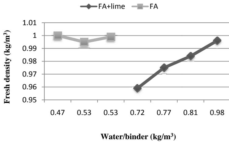
**Figure (2): Relationship between fresh density and water/binder**
