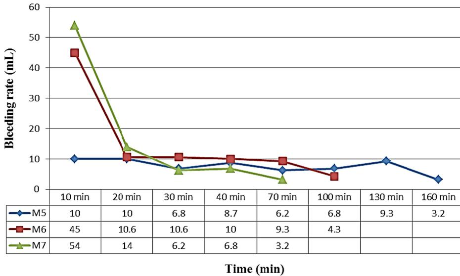
Figure (6): Relationship of bleeding versus time (M5-M7)
