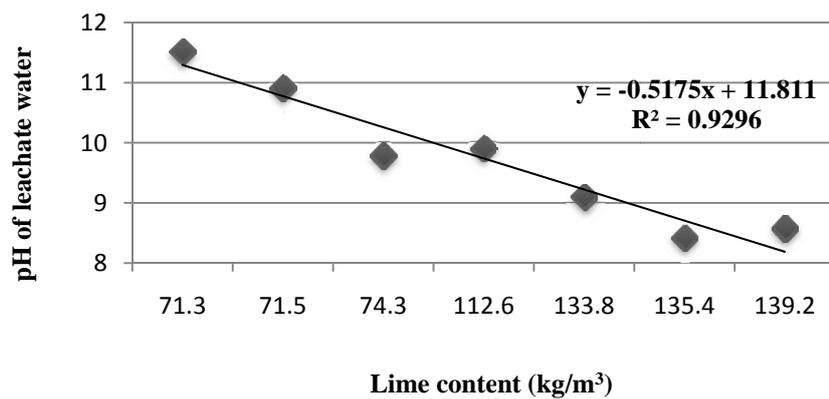
Figure (13): Relationship between pH of leachate water and lime content
