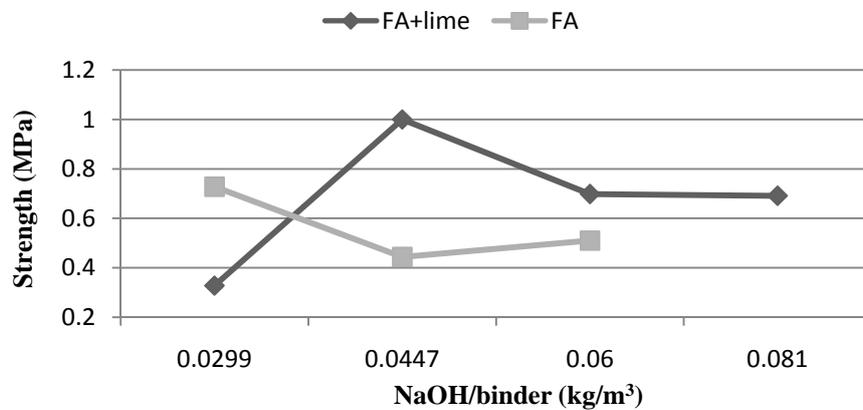
Figure (19): Relationship between compressive strength and NaOH/binder
