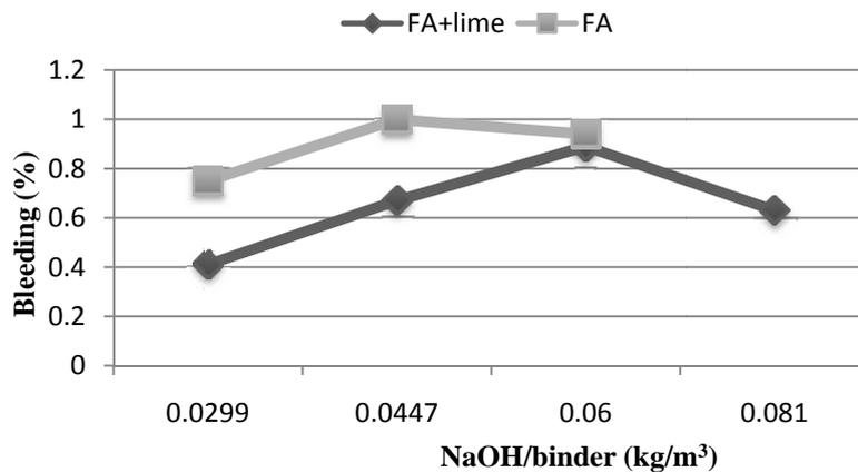
Figure (9): Relationship between bleeding rate and NaOH/binder
