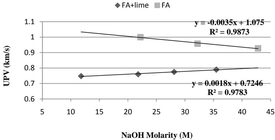
Figure (16): Relationship between UPV and NaOH molarity
