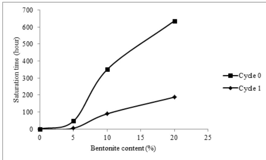
Figure (11): Saturation time vs. bentonite content
