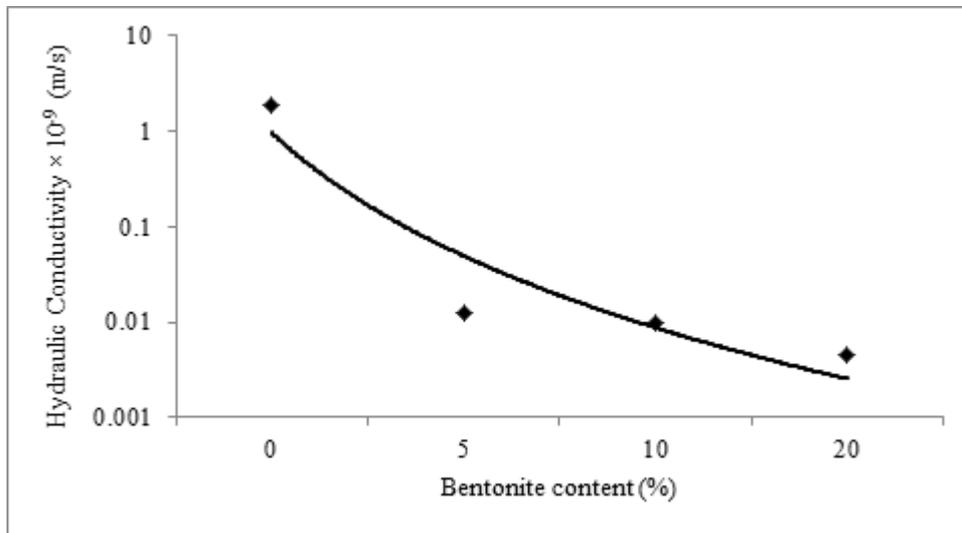
Figure (8): Bentonite content vs. hydraulic conductivity
