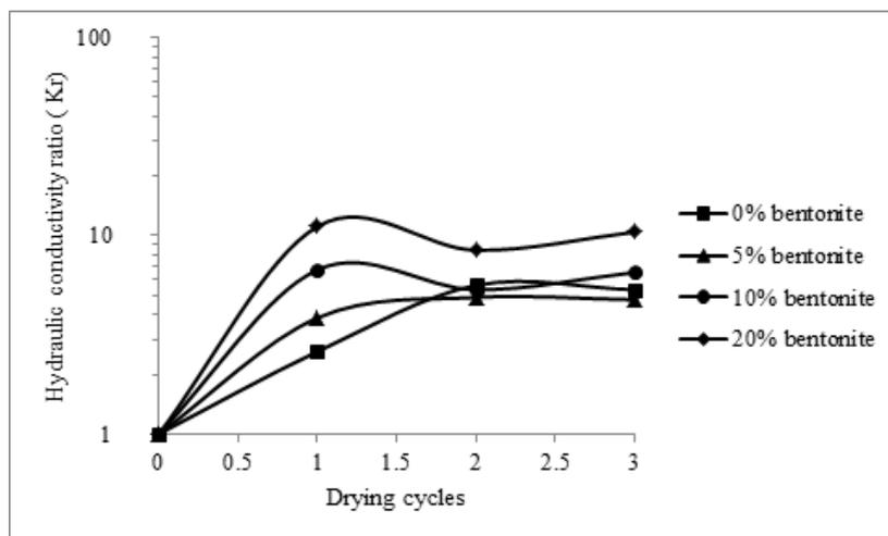
Figure (10): Hydraulic conductivity ratios vs. drying cycles
