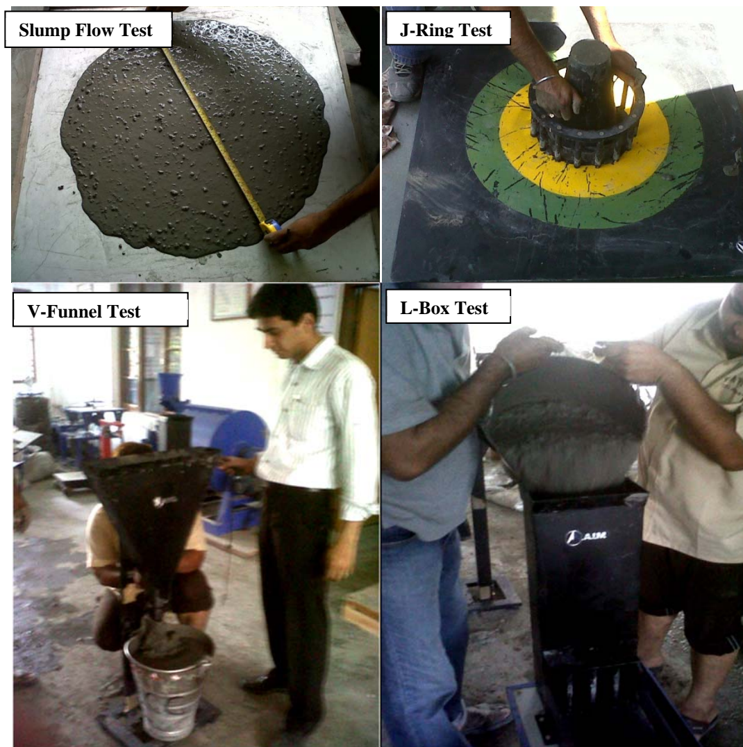
Figure (2): Workability tests conducted on SCFRC mixes
