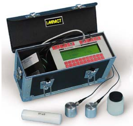
Figure (3): Ultrasonic pulse velocity tester with microprocessor
