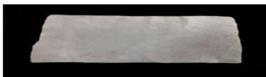
Figure 4. Non-woven geotextile reinforcement
