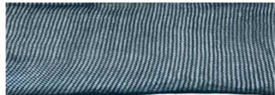
Figure 3. Woven geotextile reinforcement
