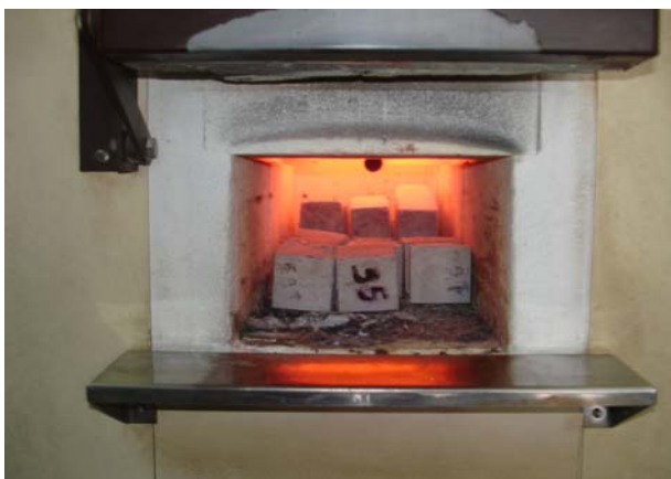
Figure (1): Specimens inside the Furnace.
