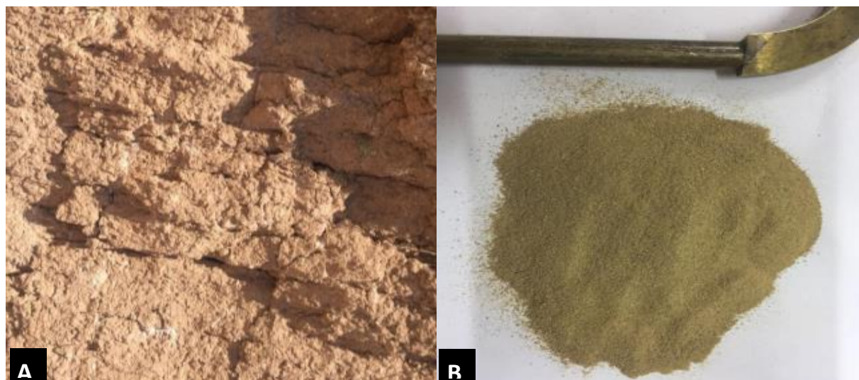
Figure (3): (A) Fine-grained clayey soil used in the study, (B) CKD from a cement factory in the Baziyan area, north Iraq
