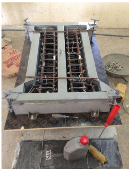
Plate (2): Steel molds and reinforcement cage
