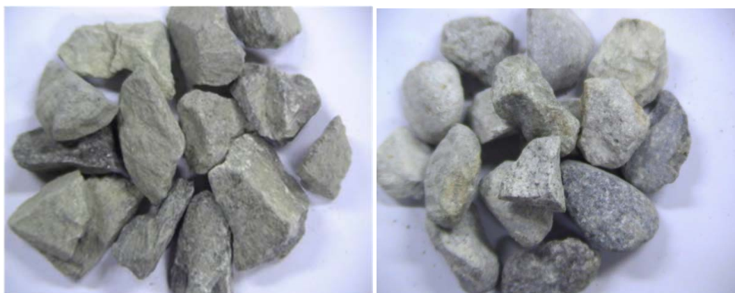
Figure (1): The coarse aggregates used in this study; (a) natural coarse aggregate (NG), (b) recycled coarse aggregate (RG)
