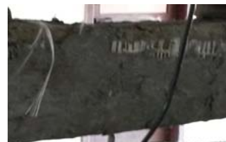
(b) Failure of beam without debonding
