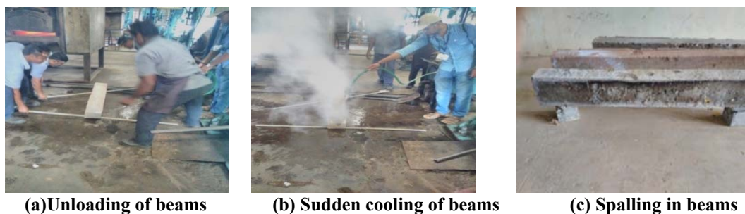
Figure (2): Beams subjected to fire loading
