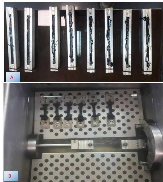
Figure (1): A) Bitumen mastic bending beam samples for the BBR test and B) Molded samples of bitumen mastic for the DT test
