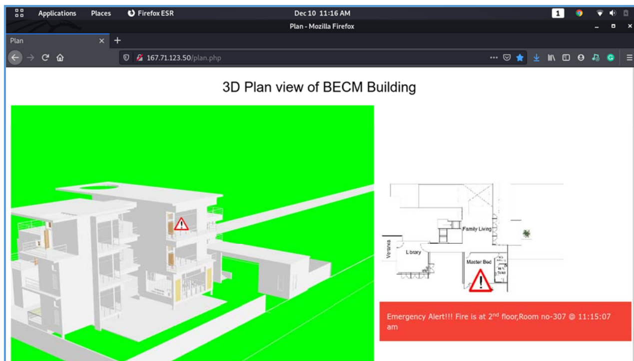
Figure (11): Automated location of fire in the building (2D and 3D views)
