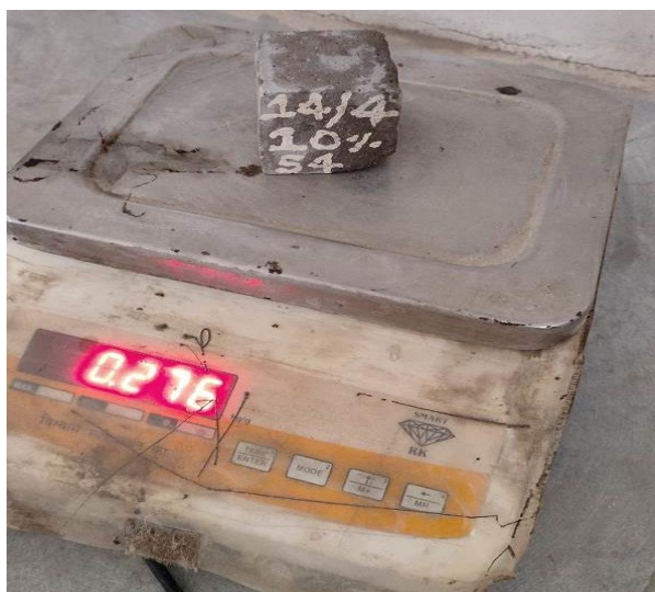
Figure (8): (a) Weighing cube after 48 hours of immersion
