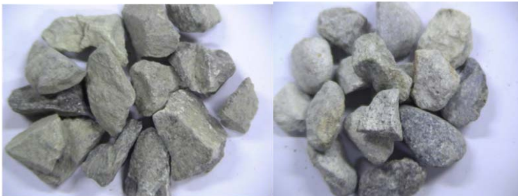
Figure (1): The coarse aggregates used in this study; (a) natural coarse aggregate (NG), (b) recycled coarse aggregate (RG)
