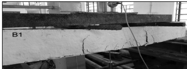
Figure (5): Yielding of bottom steel plate in composite beam B1
