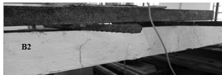
Figure (6): Ductile mode of failure in composite beam B2
