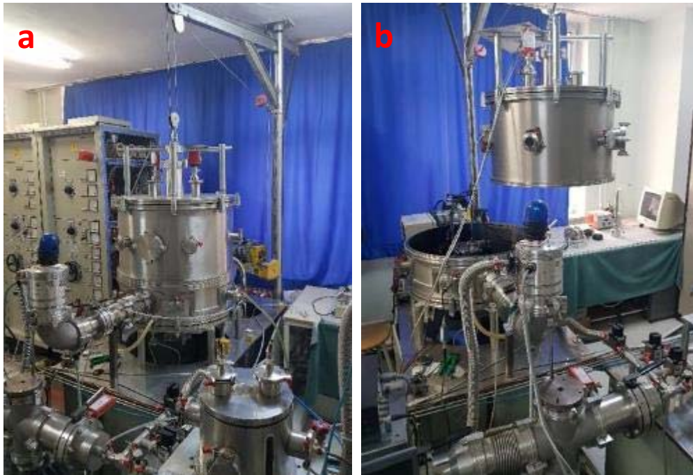
Figure (2): (a) Outside view of thermionic vacuum arc system and (b) Opening view of the system
