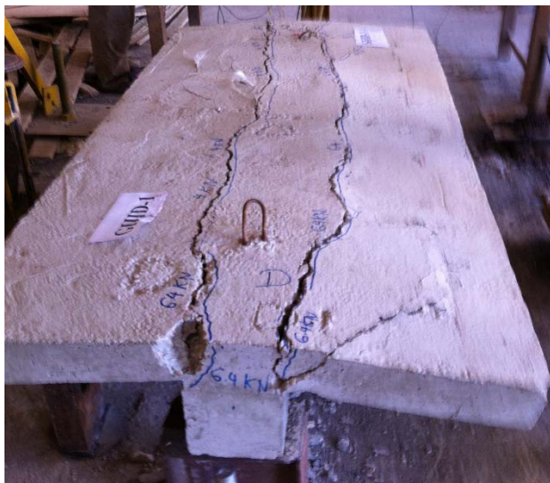
Figure (19): Crack pattern in the slab of specimen GIID-1
