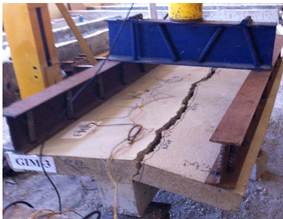
Figure (14): Crack pattern in the slab of specimen GIM-3
