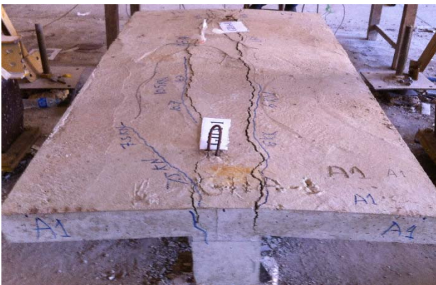
Figure (17): Crack pattern in the slab of specimen GIIA-1
