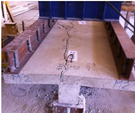
Figure (13): Crack pattern in the slab of specimen GIM-2
