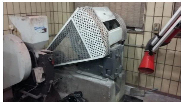
Figure (1): Grinding machine used for crushing and grading of construction waste
