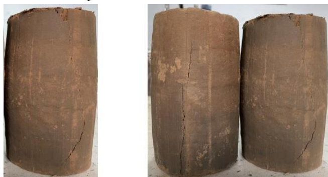
Figure (3): Failure modes of frozen sulfate saline silty clay samples after triaxial-shear tests
